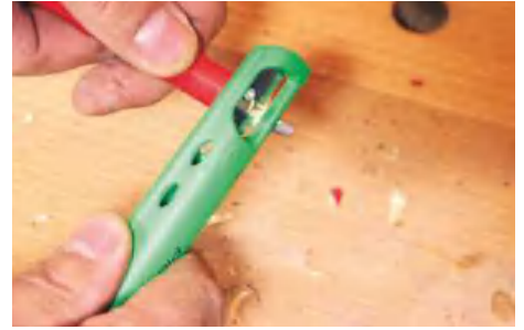
▲ A simple sharpener is used like a knife, although only suitable for right-handed use
